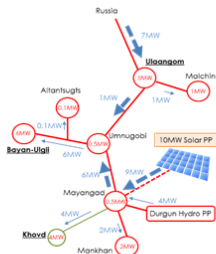
Figure 2. Load flow after 10 MWp Solar integration
