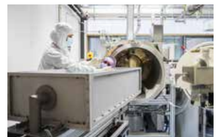
The production of highly reflective mirrors for laser applications in a clean lab. The technology is being optimized for use in laser fusion.
