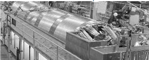
Manufacturing of first LNG CWHE bundle: Weight 275 tons Diam. 5 m, Length: 30 m Installed tubes: 600 km
