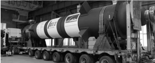
Manufacturing third CWHE for the Amur He-Plant
