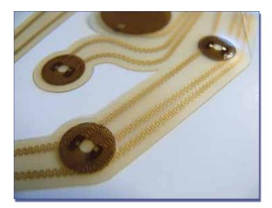
Fig. 1: Example of Polyurethane Printed Circuit Board with Meandering Shape of Conductors
