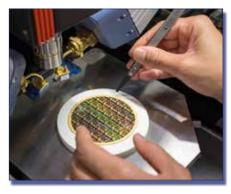
Fig. 3: On-wafer terahertz measurement setup: preparing an InP DHBT wafer for comprehensive circuit characterization up to > 500 GHz Source: ©FBH/schurian.com
