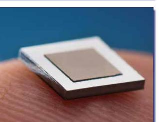
**Fig. 2:** 5 x 5 mm<sup>2</sup> silicon micropump on finger tip
