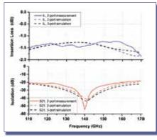
**Fig. 4:** Comparison of the measured and simulated S-parameters of the D-band RF-MEMS based SPDT switch in 0.13 µm SiGe BiCMOS technology [7].
