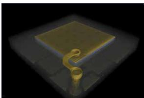
X-Ray image, 3D routing with embedded LED
