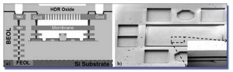
Fig. 3: The schematic cross section (a) and SEM image (b) of the WLE RF-MEMS switch [6].
