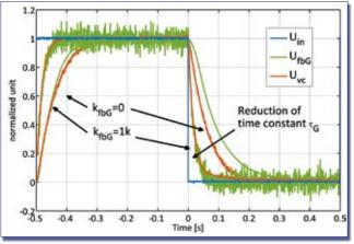
Fig. 4: Normalized step response of the optical and the electrical signals dependent of the feedback  $k_{\rm tbG}$
