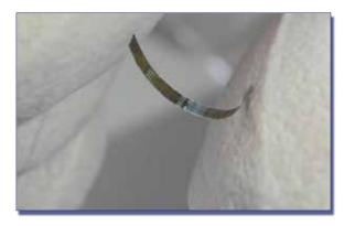
Photo of thinned and bent capacitive CMOS pressure sensors
