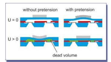
Fig. 1: Reduction of dead volume by pretension
