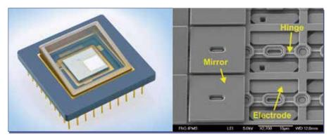
Fig. 1: Spatial Light Modulator (SLM) assembly (left) and SEM image enlargement (right)
