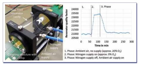
Fig. 4: Oxygen measurement with sensor system
