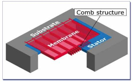
Fig. 1: Schematic view of the novel design with a comb structure.
