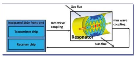
Fig. 2: Block diagram of the sensor system
