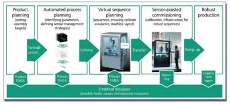
Fig. 1: Model-based machine tool chain for complex, sensor controlled assembly processes
