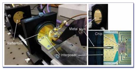
Fig. 3: Coupling between resonator and chip
