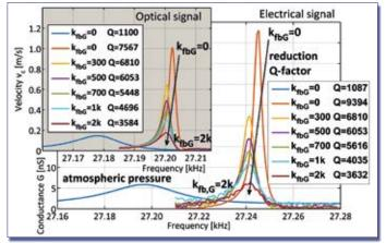
Fig. 3: Frequency spectrum of the MEMS cantilever as a function of the feedback  $k_{bG}$  resulting from the optical and electrical measurements
