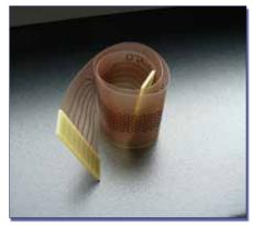
Fig. 2: TWINflex® PCB Made of Polyurethane with Partial Stiffener
