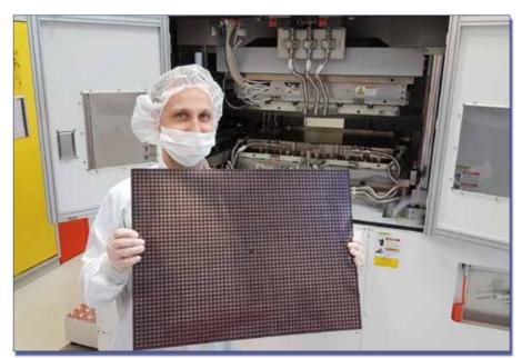
Embedded chips in molding compound Panel Level Packaging on 18" x 24" (457x305 mm<sup>2</sup> panel size)
