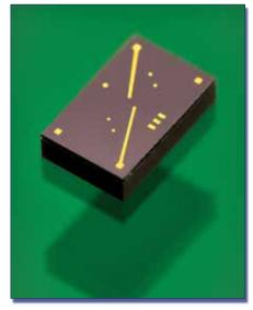
Fig.2: Wafer level packaged MEMS component
