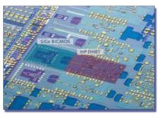
Fig. 1: Heterointegrated circuits combining the high RF output power of InP DHBT and the complexity of SiGe BiCMOS technology Source: ©FBH/schurian.com
