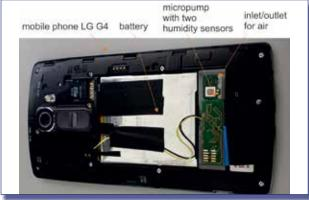
Fig. 4: Demonstrator micropump and humidity sensors, integrated in a mobile phone.
