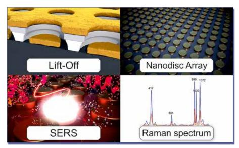
Fig. 1 (from top left to bottom right): schematic cross-section of the nanostructured resist double layer (gray & white) with deposited gold (yellow) before the lift-off step; resulting periodic metal nanodisc array on the substrate after lift-off step; schematic field enhancement in the metal nanodisc for surface-enhanced Raman spectroscopy (SERS) for molecule detection; and measured SERS spectra.
