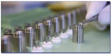
Figure 1: Assembly of micro metering pumps, Source: HNP Mikrosysteme GmbH
