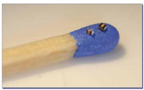
Fig.1: CMOS image sensors with through silicon vias
