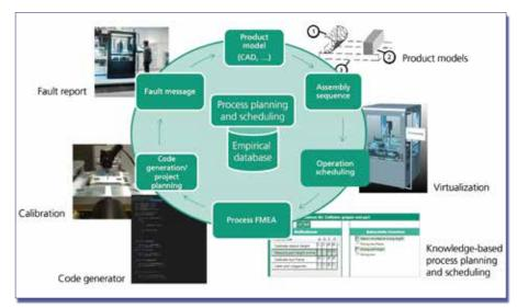
Fig. 2: Model and experience based cycle for planning complex processes
