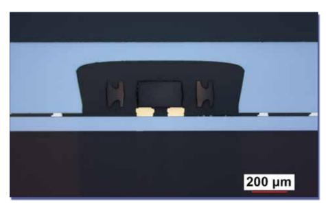
Fig.3: Hermetic bonding of TSV and cap wafers
