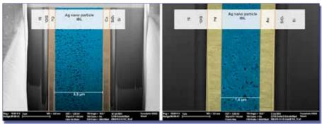
Fig. 1: SEM picture after FIB preparation of a silver nanoparticle intermediate layer between adhesion promoter Cu (left) and Au (right) after wafer-level bonding
