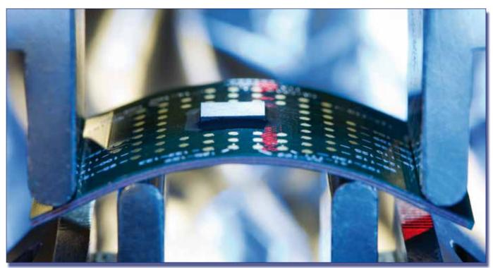
Fig. 2: PCB Module Reliability Test. © Fraunhofer IZM, Jürgen Lösel
