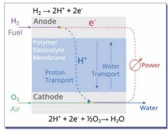
Fig. 1: Working principle of a hydrogen fuel cell.
