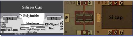
**Fig. 1:** The generic cross section of the packaged 0.25  $\mu$ m BiCMOS technology RF-MEMS switches (a) and the micrograph of K-band RF-MEMS switches before (b) and after Si cap (c) [3].
