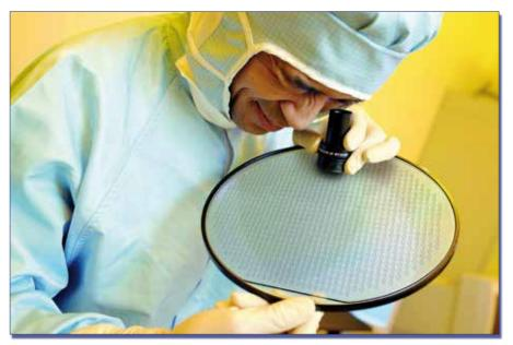
Fig. 2: SCHOTT HermeS<sup>®</sup> glass substrate wafers with hermetically sealed Through Glass Vias (TGV) are available in several glass/metal configurations, depending on the application. Via pitch and overall layout can also be configured by the customer (with the specifications of the chosen glass/metal combination). Image: SCHOTT
