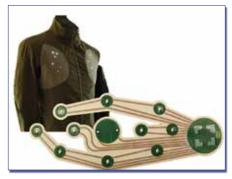
Fig. 3: Example of Use: Cyclist Jacket with Embedded Polyurethane Circuit Board (Utope, Wolfgang Langeder and Fraunhofer IZM)
