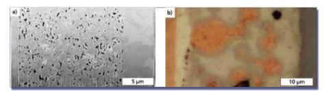
Fig. 3: Die attach interfaces. a) Sintered silver bonded at 250 °C, b) CuSn bonded at 225 °C
