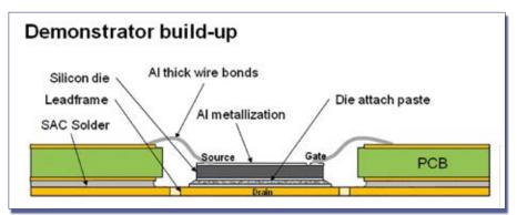
Fig. 2: Schematic built-up of a die attach sample, ready for power cycling tests
