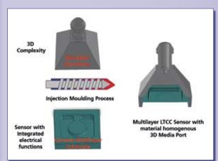
Fig. 1: Principle of the new technology approach
