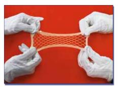
Fig. 5: Stretchable Polyurethane Based Board
