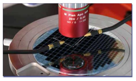
pressure stress by targeting the device inside an environmental or vacuum chamber. The Polytec MSA Micro System Analyzer has a stand-off distance that allows the researcher to characterize static and dynamic behavior under specific environmental conditions and can be easily interfaced to vacuum or pressure chambers and probe stations.
