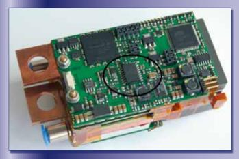
Fig. 3: CFS1000 attached to controller board of a DC/DC converter (source: Fraunhofer IISB)
