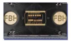
Fig. 2: A building block for THz detector modules in terahertz systems: GaN THz HEMT detector Source: ©FBH/schurian.com
