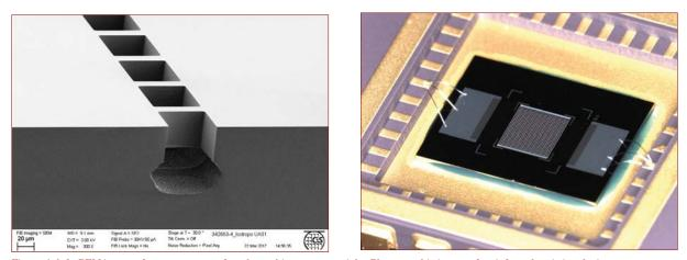
Figure 1: left: REM image of test-structure after the etching process, right: Photographic image of an infrared emitting device.
