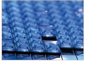
Optical Wafer level package with tilted glass windows for shifting the parasitic reflex out of the projection plane.
