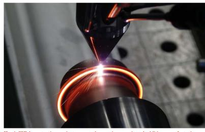
Fig. 1: EHLA: protection against wear and corrosion, repair and additive manufacturing – all with only one system technology.  $\circledcirc$  Fraunhofer ILT, Aachen, Germany
