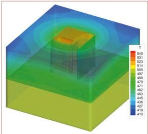
Fig.4: Simulation of the temperature distribution in a preheated LPBF process. © Fraunhofer ILT, Aachen, Germany.
