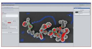
Figure 2: ZEISS ZEN Intellesis training interface - identification of individual nanoparticles. Image acquired using a ZEISS FE-SEM.
