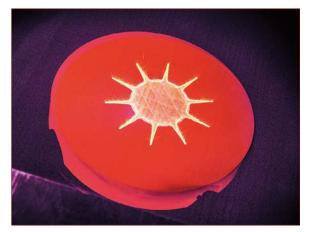
Fig.1: With up to 2.5 kW, the working plane is preheated independently of the overall height. © Fraunhofer ILT, Aachen, Germany / Volker Lannert.
