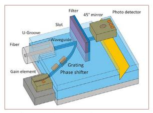
Figure 2: Illustration of Technology Platform PolyPhotonics Berlin
