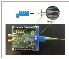
Figure 3: Assembly prototype of polymer-based tunable transmitter
