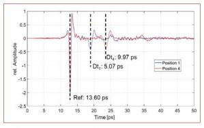
Fig. 3. Temporal THz signal (left) and the corresponding spectrum of the zirconia coating on IN 738 (right).
