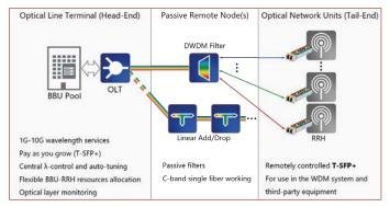
Figure 1: Mobile fronthaul enabled by passive WDM technology
