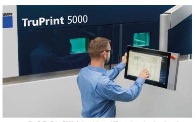
Fig. 2: TruPrint 5000: Industrial metal 3D printing using three laser beams (Source: TRUMPF)
