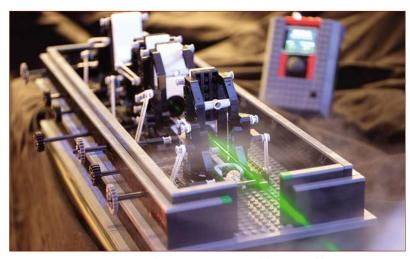
First diode-pumped, intra-cavity frequency-doubled Nd:YAG laser (DPSS) made of LEGO® bricks, Image: Prof. Dr. Mirco Imlau.
