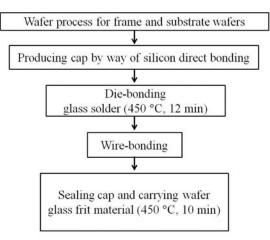
Figure 3: Flowchart of the packaging of infrared emitting devices.
