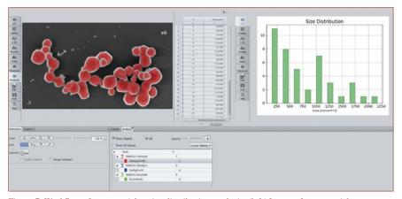
Figure 5: Workflow of nanoparticles size distribution analysis: (left) Image of nanoparticles acquired at 2kV in a ZEISS FE-SEM using the InLens detector, then segmented using ZEISS ZEN Intellesis. (right) Particle area distribution of individually segmented nanoparticles.
