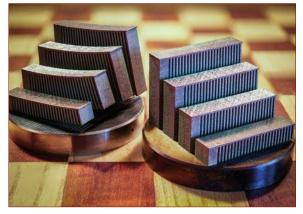
Fig.3: The component preheated with VCSEL (right) has significantly less distortion than the component not preheated during the exposure process. @ Fraunhofer ILT, Aachen, Germany / Volker Lannert.
