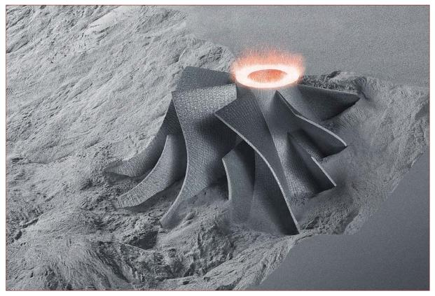
Additive Manufacturing using Laser Metal Fusion (LMF). Image: TRUMPF Gruppe
