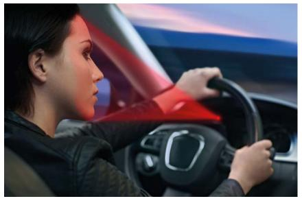
For driver monitoring the IREDs illuminate the driver precisely so that a camera can capture the drivers' status (drowsiness, distraction) and pass this information to the system.
