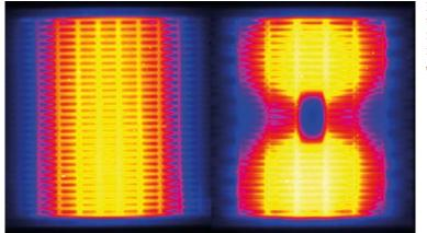
Figure 2: Lock-in thermographic images of different infrared emitting grid structures.
