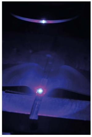
Welding of a copper sheet with 450 nm wavelength ©Laserline
