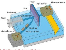
The PolyPhotonics Technology Platform © Fraunhofer HHI
