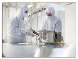
Fig. 3: Assembly of a space telescope with free-form optical components. ©Fraunhofer IOE
