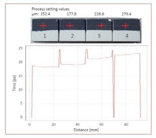
Fig. 2 Top: Photo of zirconia coated IN 738 sample (89 mm x 19 mm x 9 mm). Upper half is additionally sprayed with graphite. Bottom: time delay profile over the indicated dashed line of the top picture
