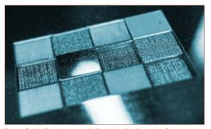
Image 3: Application example for "mixed pulse trains": matt areas were ablated with 100x - 1000x 400 fs pulses, reflective areas where smoothened with 20x 12 ns pulses.
