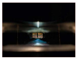
Pathogens and resistance genes in surface waters can by detected using a plasmonic micro-array and hyperspectral imaging. © Sven Döring, Leibniz-IPHT
