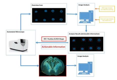
Figure 1: The general concept of Actionable Information – Use Image Analysis and Machine-Learning to guide the next acquisition steps in automated workflows or for the final image analysis
