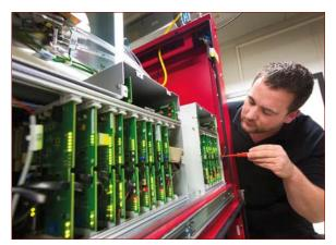
Production of Laserline diode lasers
