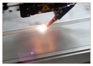
Brazing process with triple-spot module
