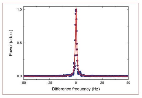
Figure 4: Narrow-linewidth lasers are key for applications like optical clocks. By locking to a high-finesse optical cavity, the linewidth of external cavity diode lasers can be reduced to the 1 Hz level. The graph shows the optical beat signal between two independent, cavity-stabilized TOPTICA diode lasers at 1162 nm.
