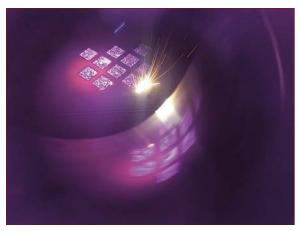
Fig.2: Exposure with simultaneous VCSEL preheating. © Fraunhofer ILT, Aachen, Germany / Volker Lannert.
