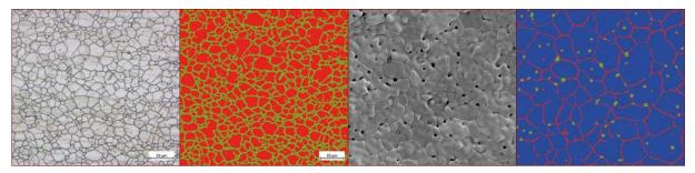
Figure 6: (left) Nickel Alloy 600 after metallographic preparation and electro etching. Brightfield imaging on a ZEISS Axio Imager Z2.m. (half left) ZEISS ZEN Intellesis segmentation of this image, showing grains in red and grain boundaries in green. (half right) Zirconia in the as-received condition, secondary electron imaging at 1kV at 30Pa in a ZEISS Sigma 300 VP. (right) ZEISS ZEN Intellesis segmentation of this image, showing grains in blue, grain boundaries in red, pores in green.
