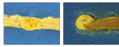
Welding of 34 stacked copper foils (each 11  $\mu$ m) in butt welding (left) and edge welding configuration (right) ©Laserline
