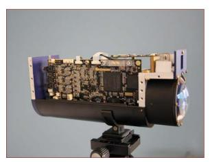
3D camera with FPGA-based electronics.
