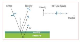
Fig. 1: Schematic of the THz pulse-echo method illustrating their reflectivity at interfaces. The reflectivity depends on the refractive indices of the layers.
