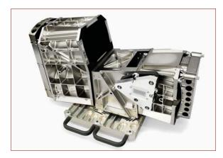
Figure 2: Complete optical system of DESIS consisting of a Three-Mirror Anastigmat telescope with a focal length of 320 mm, and a corresponding Offner type grating spectrometer for observing the ecosystem of the Earth's surface. © Fraunhofer IOF
