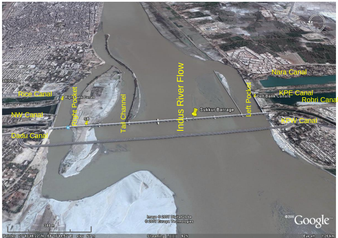
Figure A1.1. Plan View of Existing Barrage and River Training Works
